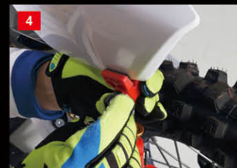
Attach sag checker clamp on side panel or rear fender.
