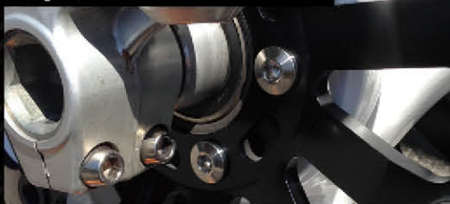
Front DISC BOLT Flange Bolt 10 mm - M8 x 22
