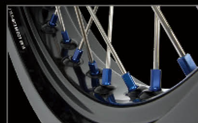
Z-WHEEL aluminum nipples and stainless steel spokes are used. The front 16.5-inch wheel uses cross-spoke to minimize calliper / spoke interference.
