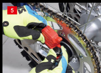
And attach sag checker body on swing arm by hooking hook into axle shaft hole.
