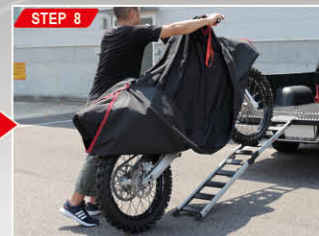
Wrap a tie-down soft hooks around the handlebar then load on a truck.
