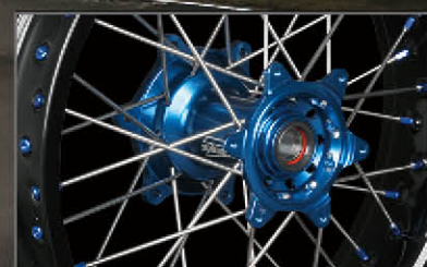
ASTELIGHT HUB, which is ultra high precision cut aluminum, achieves a light weight product compared with genuine parts. All internal parts such as bearings are press-fitted.
