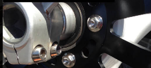
Front DISC BOLT Thin Head 10 mm - M8 x 22
