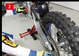
Check length between swing arm axle to rear wheel axle
